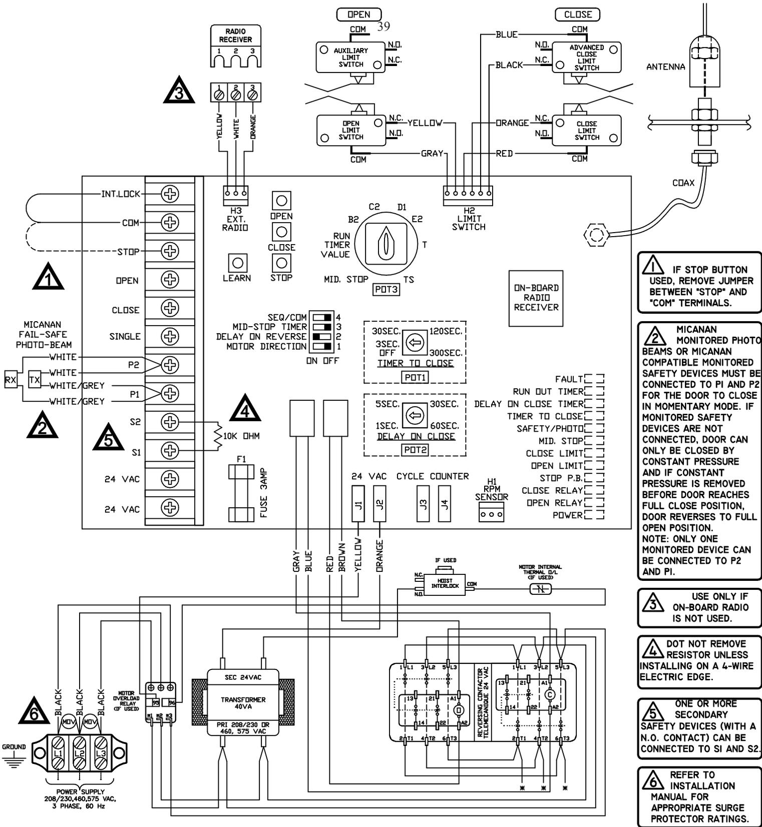
**1** IF STOP BUTTON USED, REMOVE JUMPER BETWEEN "STOP" AND "COM" TERMINALS.
