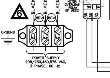
**3- PHASE WIRING DIAGRAM**
