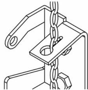
2. **If operator is supplied with optional floor level disconnect lever:** Pull disconnect lever downwards and lock in place by bending lever around bracket lip as shown.
