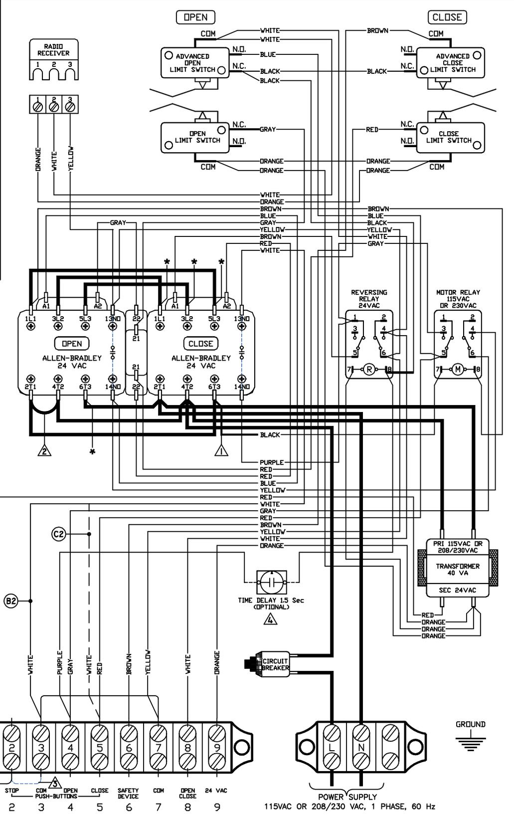
FOR 220V: REMOVE BLACK WIRE FROM C6 AND PLACE ON O4
