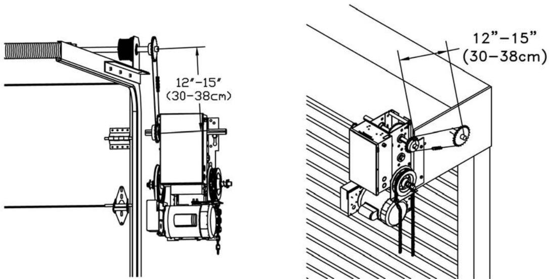
**Note:** Bracket mounting applications should be specified at time of order. To convert operator to bracket mount application, invert frame feet towards interior.
