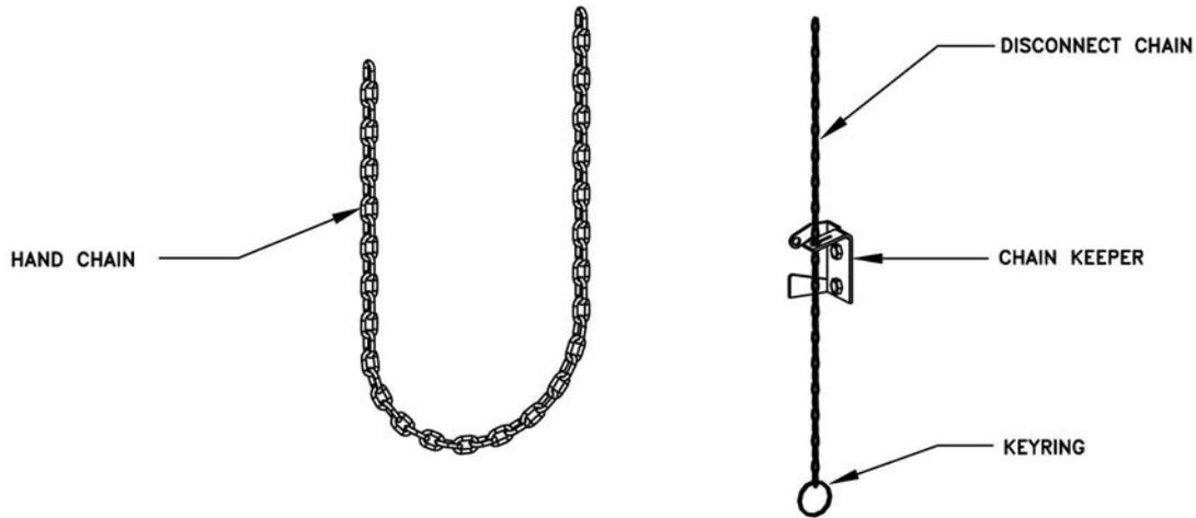
12. If an **optional** floor level disconnect lever was ordered in lieu of the chain keeper, mount to wall with suitable hardware. Attach both chains together using keyring provided. Allow disconnect chain to be slightly slack when lever is in the up position.
