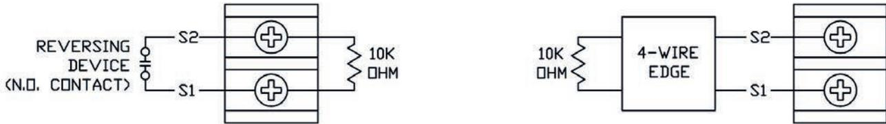
**CONNECTION OF EXTERNAL SINGLE-BUTTON DEVICE**
