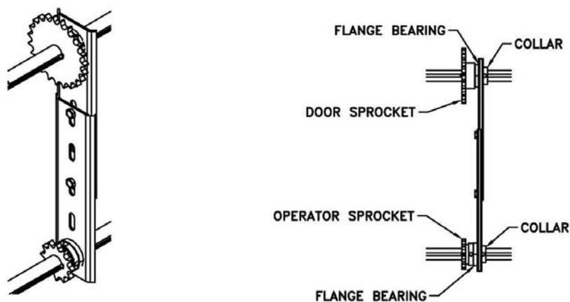
7. Install drive chain over sprockets, cut to a suitable length and connect with connecting link.
