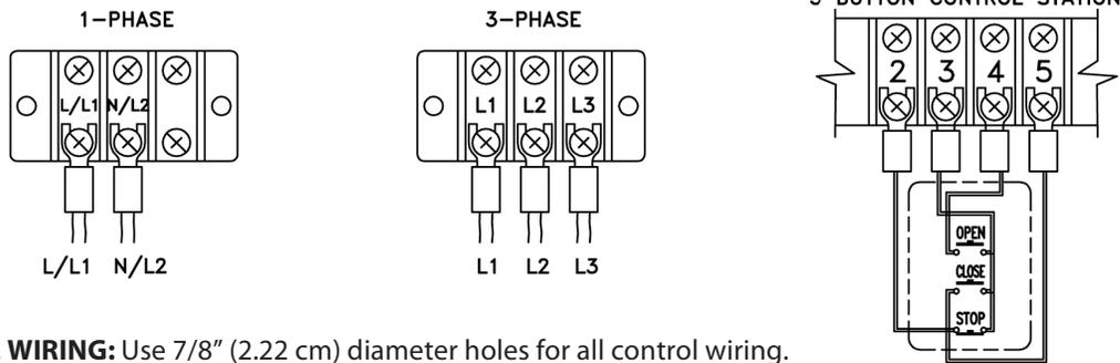
**CONTROL WIRING:** Use 7/8" (2.22 cm) diameter holes for all control wiring.
