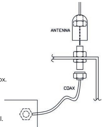
Note: Do not route coax cable near any moving parts of the operator. If necessary, secure coax wire away from any moving parts.
