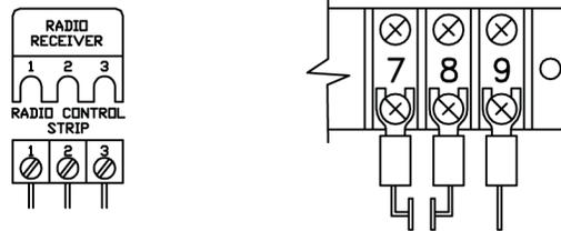
4. **Single button open/close device:** Wire to terminals 7 and 8 on control terminal strip.
