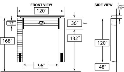
Generally designed to suit 8' wide x 10' high openings. The series D300 is used on higher door openings when a variety of trailer heights are being serviced.
