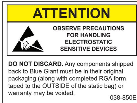
1. Prior to handling PCBs, wear a static grounding wrist strap and clip it to an electrical ground. The metal plate on the inside of the wristband must be in contact with the wearers skin.
